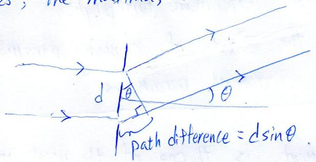
Given separation between the  $m$ -th maximum and the  $(m+10)$ -th maximum on the screen  $\Delta = 7.5 \text{ mm}$ ,  $d = 0.4 \text{ mm}$  and  $L = 600 \text{ mm}$ . We want to calculate  $\lambda$ .
